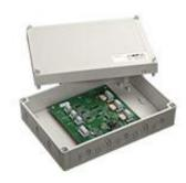
The Interface input / output unit is to enable simple interfacing between the fire alarm system and other equipment such as Basement mechanical ventilation fans, fire escape pressurization systems or access control systems.
